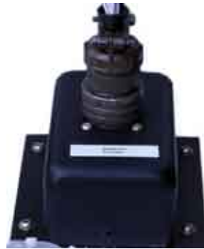
Windshield Temperature Controller
