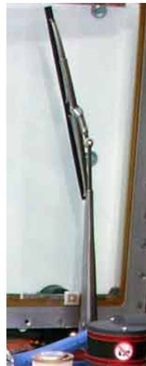
Wiper assembly shown in the parked Position
